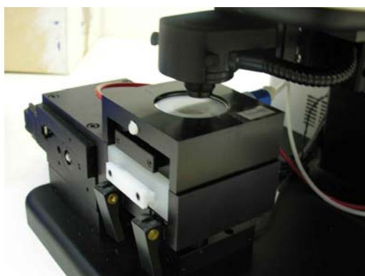
Figure 2. The new sample chamber mounted within the motorised stage of the UP-213 Laser ablation system.
