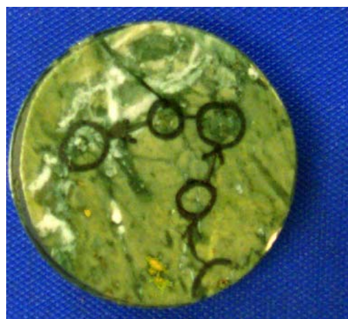
Figure 4. A rock sample set into an epoxy mount.
